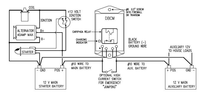
The start or crank battery should be permanently connected to the alternator output. The auxiliary or trolling battery and crank battery are connected in parallel through the DBCM-40A relay only when the alternator is charging.
