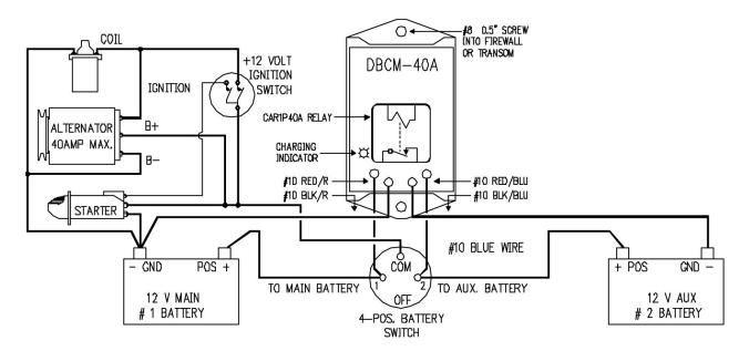
The alternator output should be continuously connected to battery #1 thru PERKO switch. Both batteries are connected in parallel through the DBCM-40A relay to receive charging current only when the alternator is charging.
